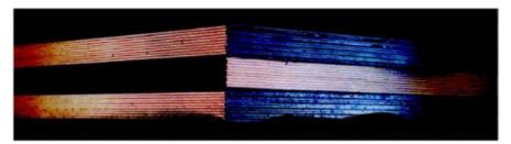
Figure 5.11-1 Three Superlayers Showing Alternating Layers Of Lead Foil And Scintillating Fibers And Alternating Superlayer Orientation
