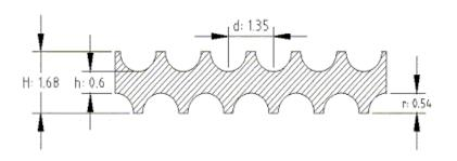
Figure 5.11-2 Individual Lead Foil Profile (Dimensions in mm)
