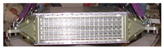
Figure 5.11-4 View of the ECAL showing the Side Panel grid prior to the installation of the PMTs
