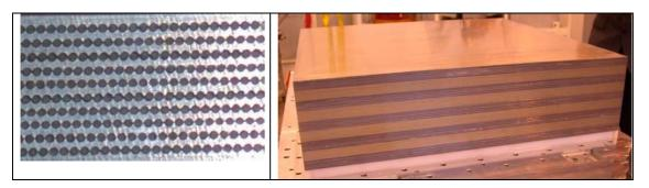
Fig : detail of the lead/scintillating fiber sandwich (left) and (right) pancake before assembly in the mechanical support structure.
